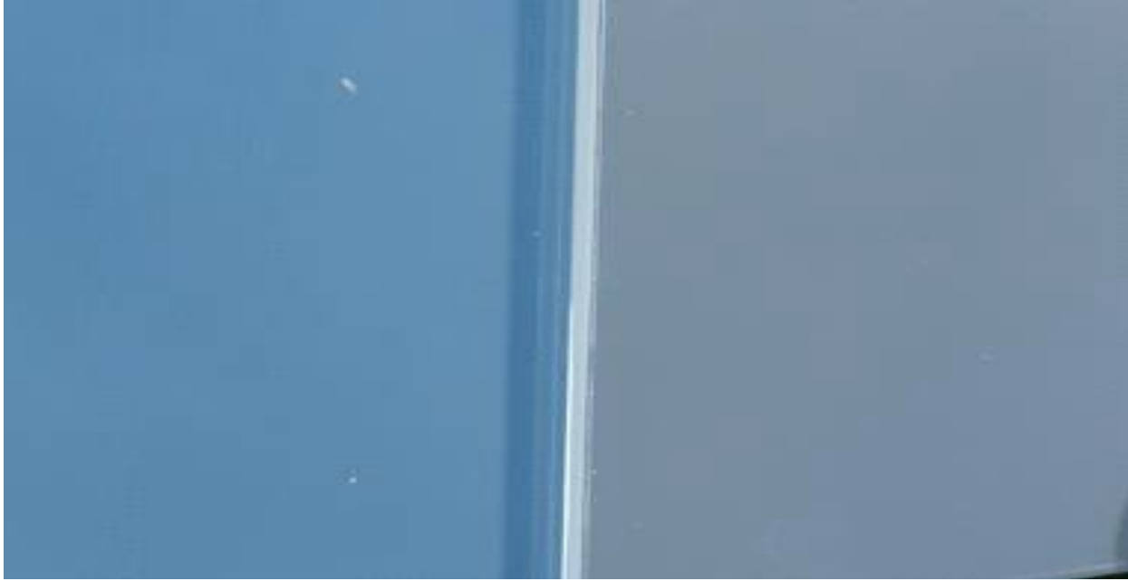
Sputter coat IG reflected color of a grey sky. The same sky reflected in adjacent clear glass IG
